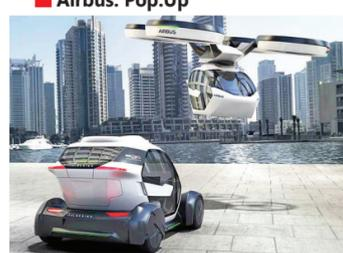
Best known for its double-decker A380 jet, Airbus premiered its solution for urban transit at Geneva international motor show in March. The Pop.Up consists of a carbon-fibre passenger capsule that functions as a two-seater electric car when attached to a chassis, or as an aircraft when a drone is summoned by smartphone to remove the capsule from the chassis.
