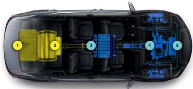
Electricq-System Existing Hydrogen Fuel Cell Existing Electric Car Engine and Power Control 1 Electricq-Fuel Tank 2 Electricq-Switch 3 Fuel Cell Stack 4 Motor 5 Power Control Unit
